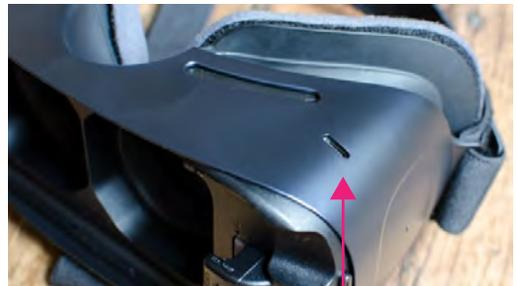
*Plug the cord into the port on the underside of the headset*
